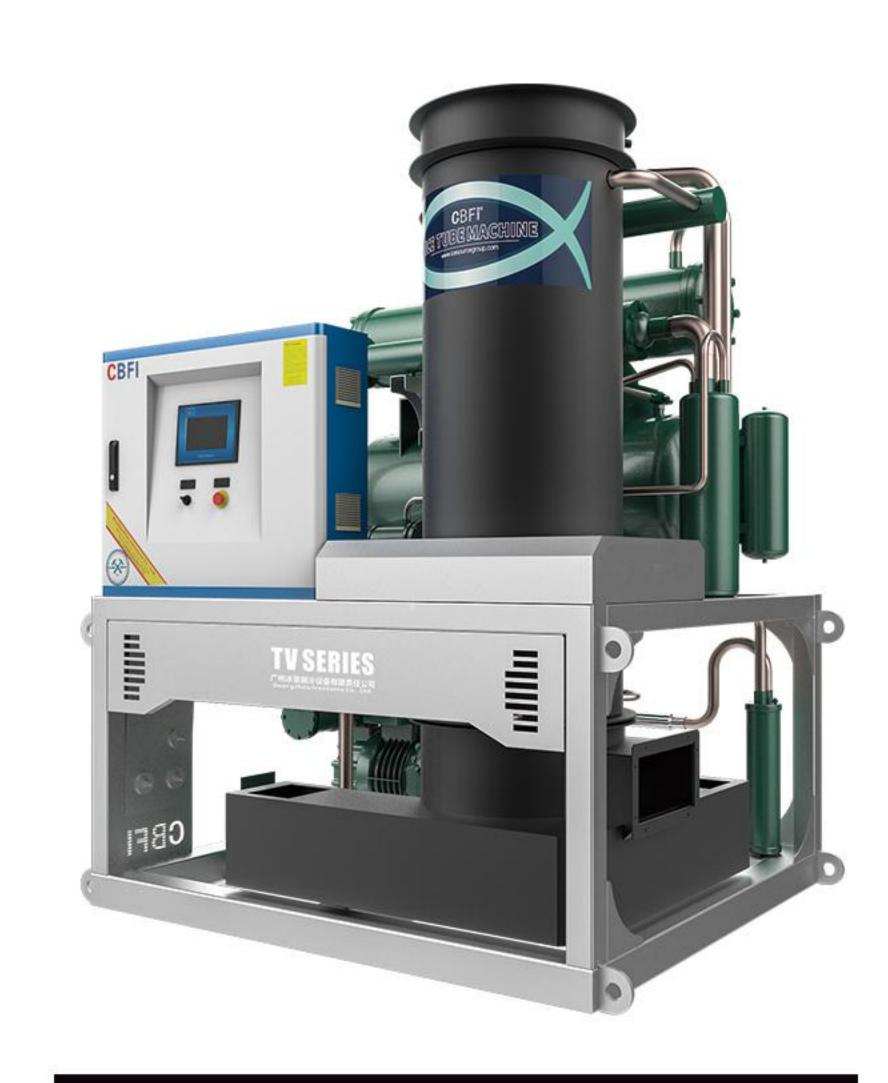
Ice Making Capacity: 1Ton/24h Compressor Rated Power: 3KW Circulating Water Pump Power: 0.37KW Cooling Water Pump Power: 1.1KW Cooling Fan Motor Power: 0.18KW Ice Cutter Motor Power: 0.75KW Ice making machine size: 1100x900x1780 (mm)
